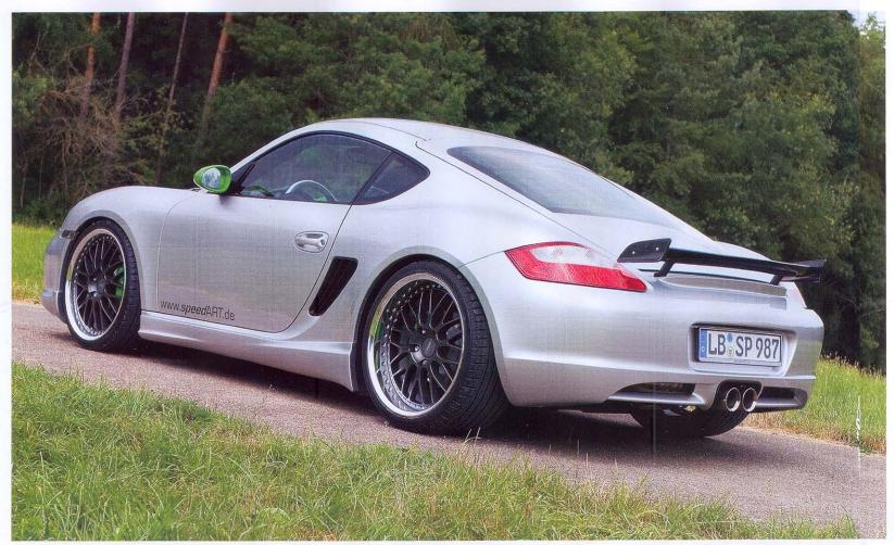
325bhp and 269lb ft of torque, 30bhp and 18lb ft up on the standard Cayman S and all but identical to the basic 997 Carrera (325bhp and 273lb ft). The exhaust itself is a combination of modified manifolds, sports cats and sports silencer, coupled to a pair of circular exhaust tips.
