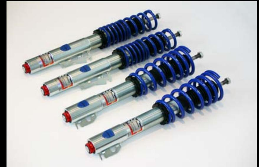
Coilover suspension setup „Race-Allround“ with PASM
